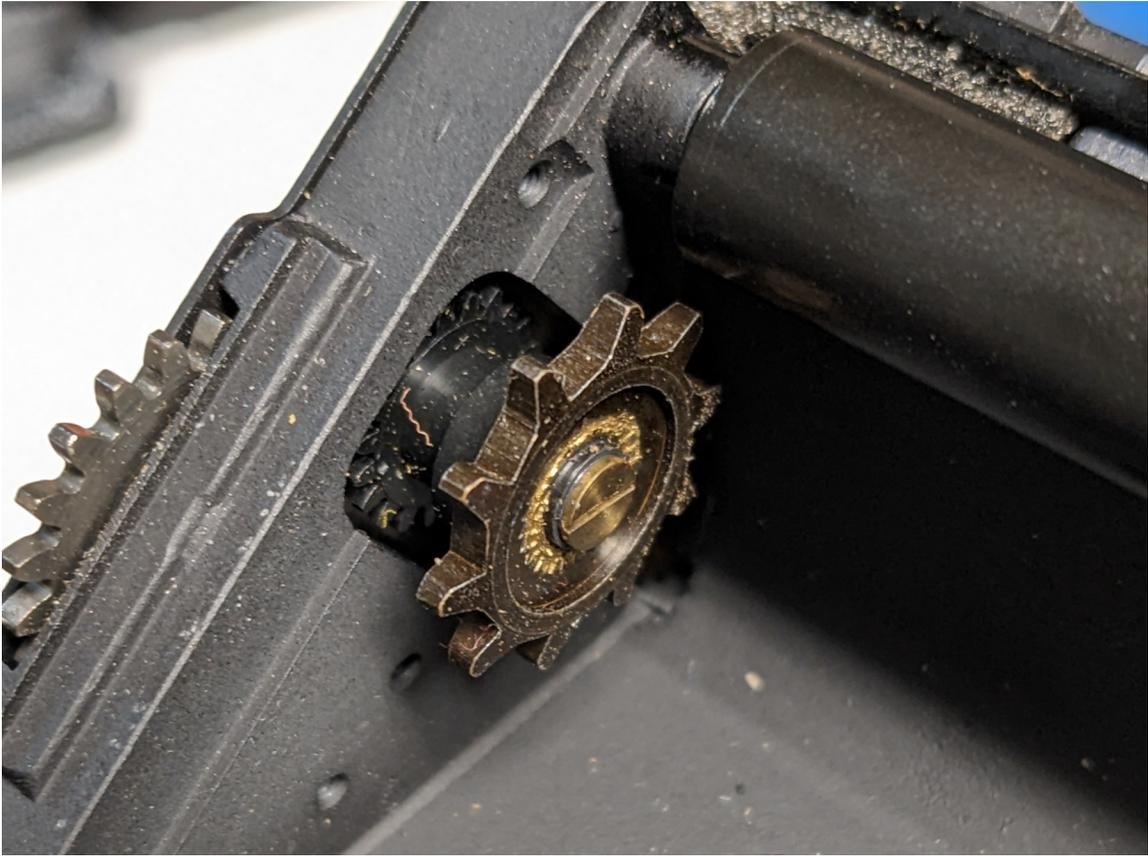
3. Use a bench grinder (best), rotary tool with grinding or cut-off bit, or diamond file to grind off all sprocket teeth. The goal is to produce a round wheel with no protrusions.
