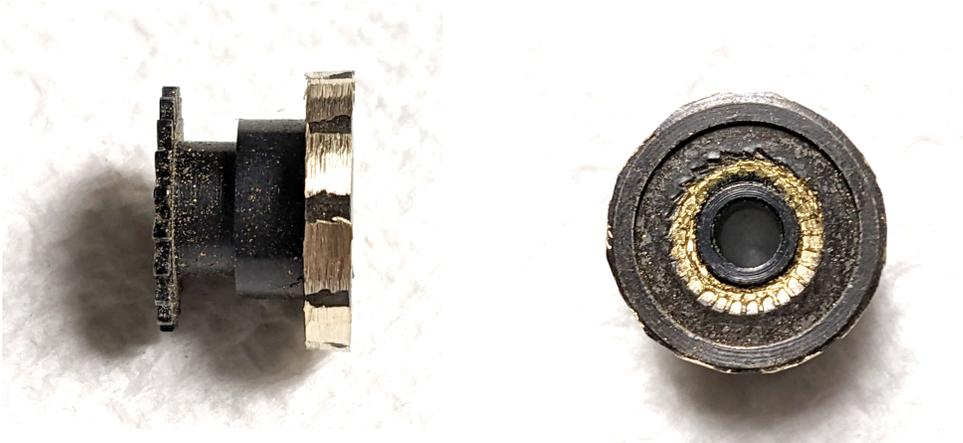
4. Press fit the Mercury plastic ring around the wheel. If it doesn't fit, grind a bit more off the wheel until it does. If it ends up fitting too loosely, fill any gaps with glue. Otherwise, no glue is necessary: ideally this should be a tight friction fit.
